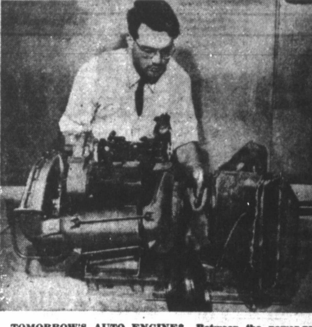
TOMORROW'S AUTO ENGINE? Between the power-producing section (left) and the power output section, there's no mechanical connection. There's no shifting—and no stalling, either.
