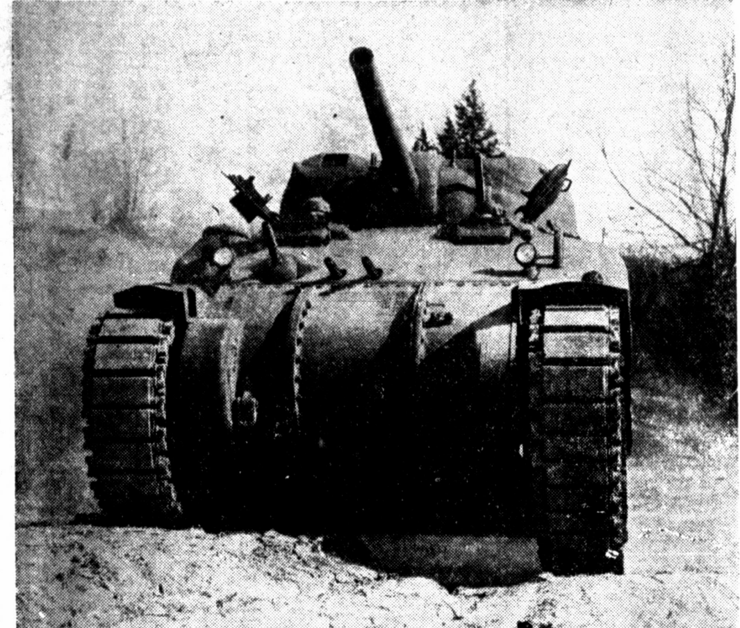
ARMY'S NEW RIVETLESS TANK GETS GUNS—Thundering around a ridge at Ft. Knox, Ky., testing ground comes the army's new rivetless medium tank complete with 75 mm. gun and a battery of machine guns. The M-4 has an all-cast body and mounts its big gun on revolving turret in center instead of lower down on the right side as on the M-3 tank.
