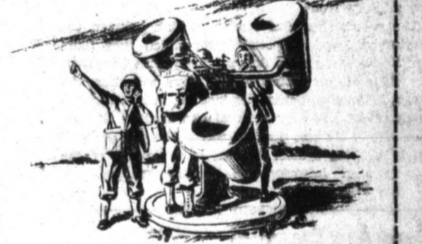
These big "ears" are the sound-scouts of the anti-aircraft units. They amplify the sound of approaching planes, locating them and determining their direction miles away.
