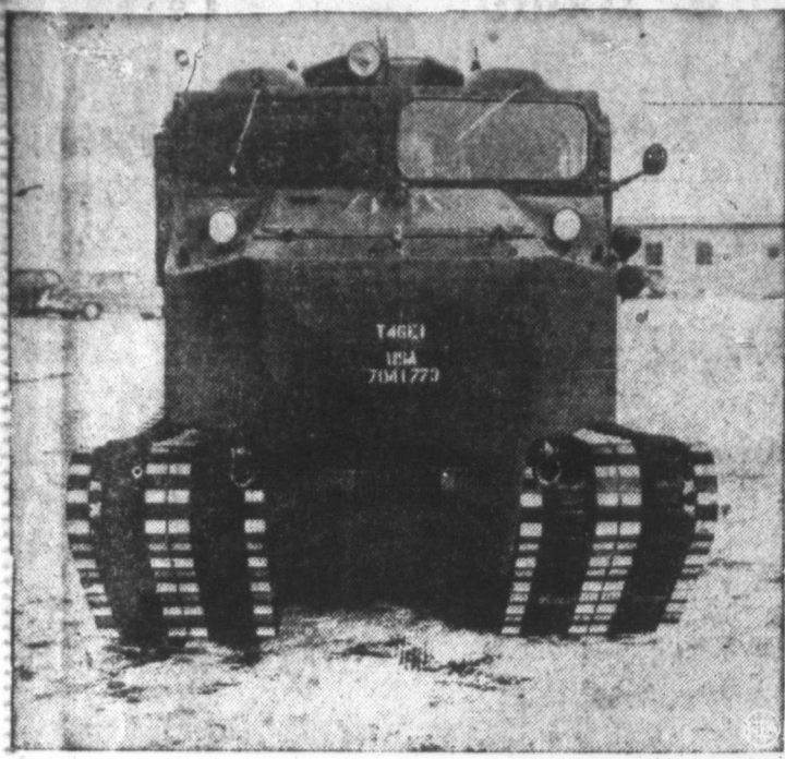
MEET THE ARMY'S "OTTER"—At home on land or sea in any climate is the "Otter," the Army's new amphibious cargo vehicle. Run by a two-man crew and carrying its own armament, the "Otter" can make 30 miles an hour on land. It is extremely maneuverable on land or afloat, can turn completely around within its own length and in water can reverse course by use of one of its two churning treads. (Dept. of Defense photo from NEA-Acme.)
