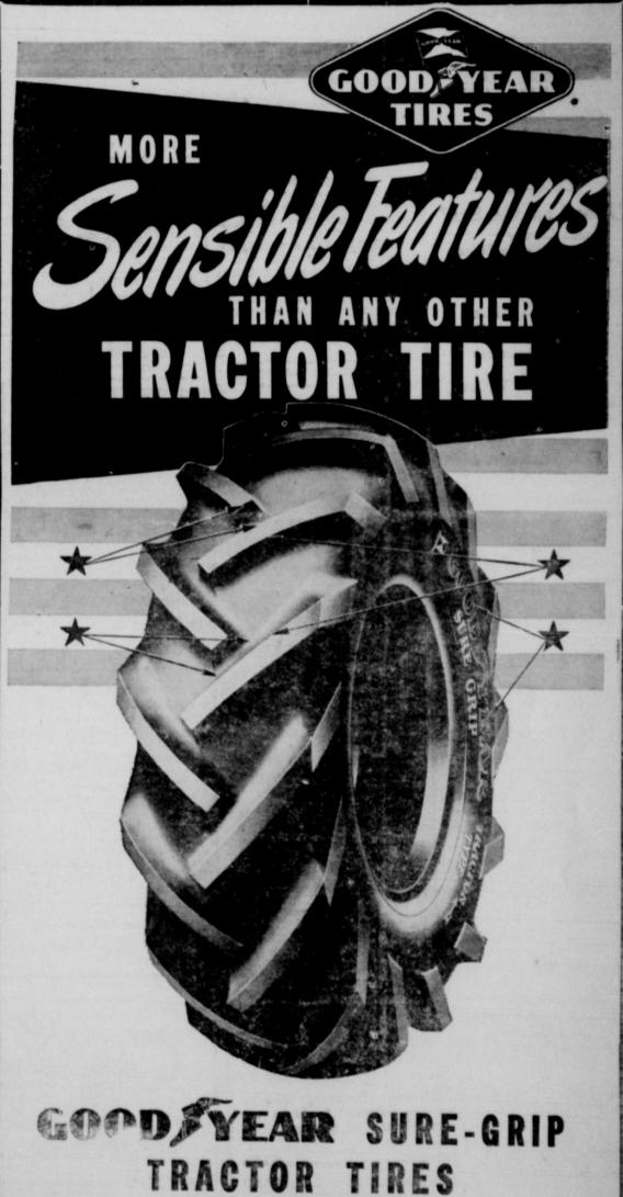
Designed for traction. Husky, field fighting lugs g-r-i-p and p-u-l-l through sand, clay, soft loam, mud and any soil condition. O-P-E-N C-E-N-T-E-R design adds extra fast self-cleaning, eliminates mud traps. Solid buttressed base protects against lug tear and lessens wear. Even spacing provides smooth pulling power, no jerks, fewer
