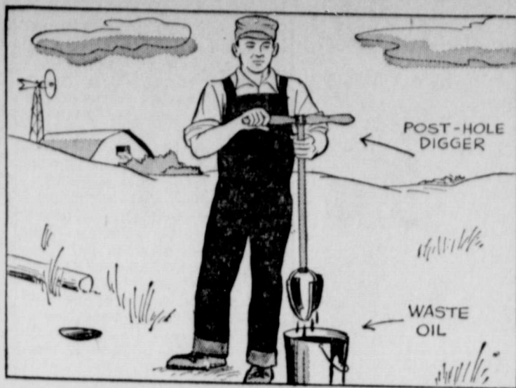
AN OIL FILM ON A POSTHOLE DIGGER prevents sticking of heavy clay and gumbo soil and makes the soil slip off easily when digger is lifted from hole. Dip digger regularly in bucket of waste oil.
