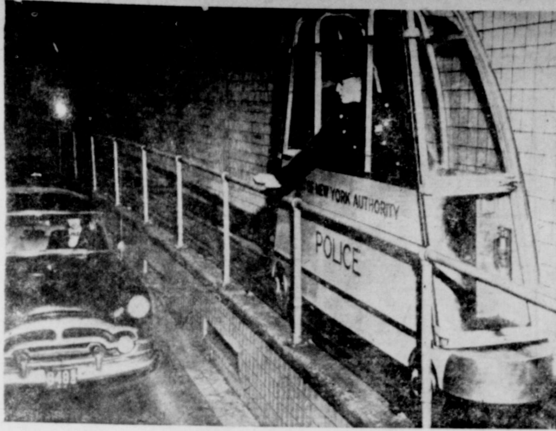
TUNNEL PATROL . . . Police use electric car to direct traffic in New York city's Holland tunnel. It has transparent plastic body, weighs 1,300 pounds and travels 12 mph.
