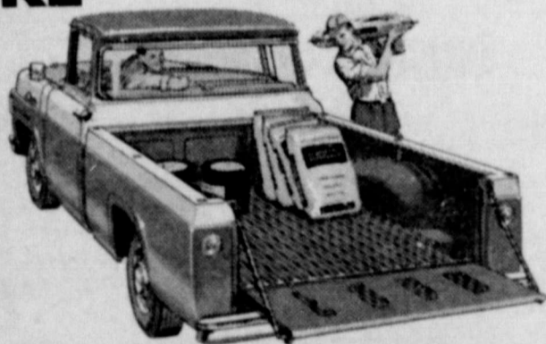
'59 Ford Styleside is roomy—and rugged! Wrap-around rear corners with rigid box girder type construction strengthen both body and tailgate.
