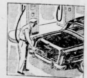
CENTER-FILL FUELING - prevents hose marks, and makes "filling up" easier from either side of gas 1 ump. Shorter gas filler pipe gives you trunk space for an extra suitcase.
