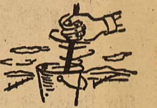
4. Break up cores or slices and mix well in bucket. Take a sample from bucket and place in a soil sample bag.
