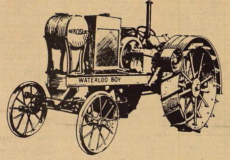
Shipping Wt. 5700 Lbs. HP - 12 Drawbar - 25 Belt - @ 750 RPM 2 Speed Straight Spur Gear Transmission
