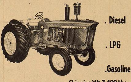
Shipping Wt. 7,400 Lbs. HP - 73.4 Drawbar - PTO - 84 @ 2,200 RPM Gears - 8 Speeds Forward - 3 Speeds Reverse
