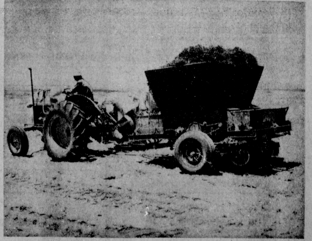
PLANTING — Second phase of getting a Bermuda grass pasture is placing the sprigs in the ground with a sprigger, shown being done here by two men from the High Plains Research Foundation at Halfway. One is seated in front of the sprigger and is hand-feeding the grass through the machine. (Journal Photo and Engraving)
