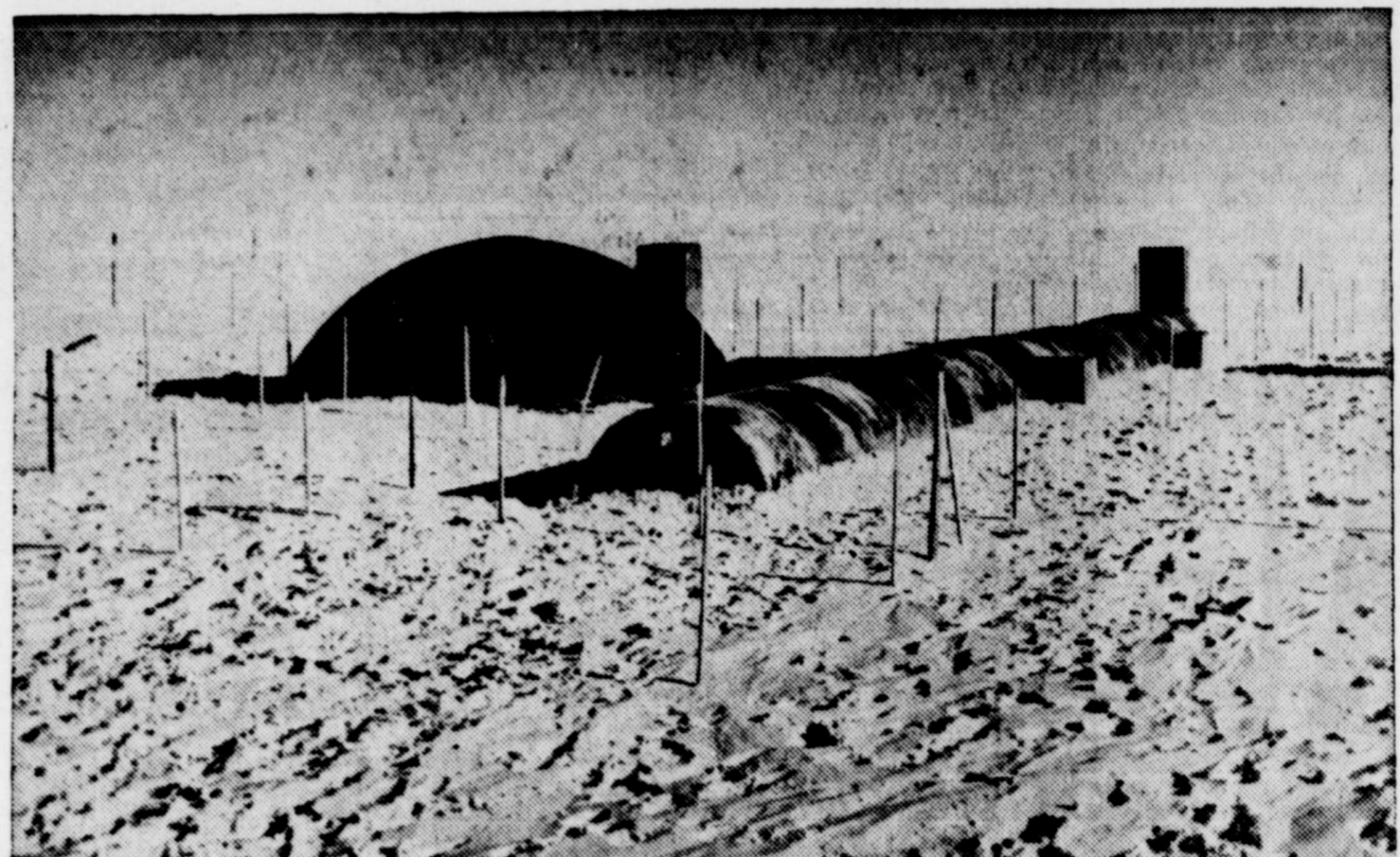
TESTING DRIFTING SNOW , engineers concerned with its effect on a proposed replacement South Pole station have set out this one-tenth scale model a half-mile from the present station. Geodesic dome is only five feet high, but actual structure will be nearly 53 feet tall, housing three separate buildings.
