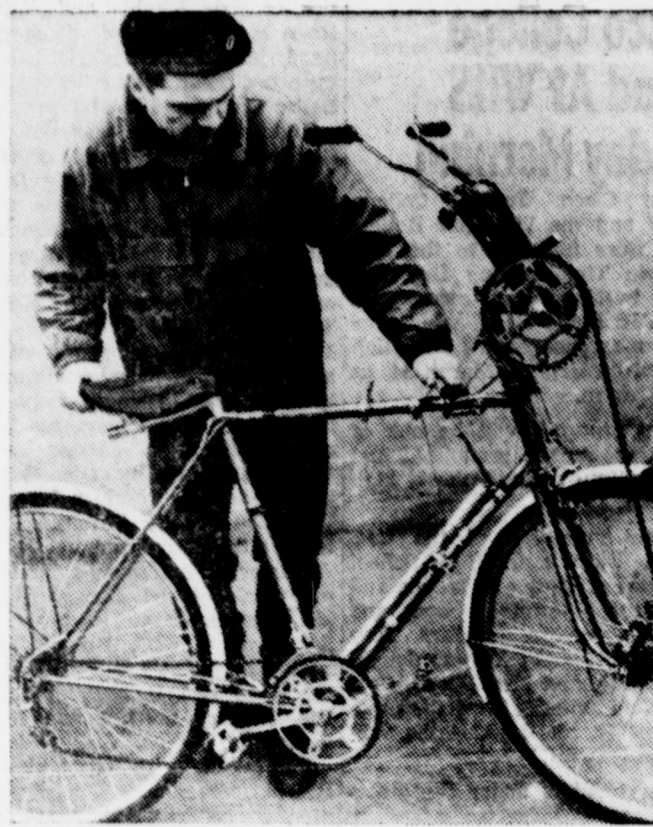
FRONT-WHEEL DRIVE is the new departure in bicycles in the Soviet Union. Leonid Dutoy, researcher at Gorky University at Kharkov in the Ukraine, developed the front-wheel mechanism operated by the hand movements that enables rider to climb steep inclines and cover rugged terrain with ease. A Kharkov plant is considering producing the bike for public use.
