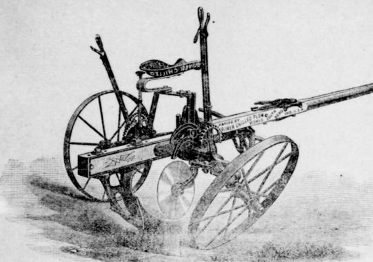
No Neck Weight, no Side Draft, no Landside to Cause Friction and Heavy Draft Allthe Weight carried on the Wheels
