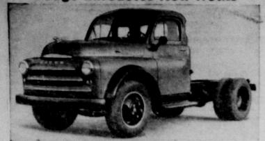
Among the 248 basic gross vehicle weight chassis models just announced in the new Dodge "Job-Rated" truck line is this B-1-H tractor of 128-inch wheelbase, 15,500 pounds gross vehicle weight (1½-ton nominal rating) and 28,000 pounds gross train weight. The trucks have many new features.
