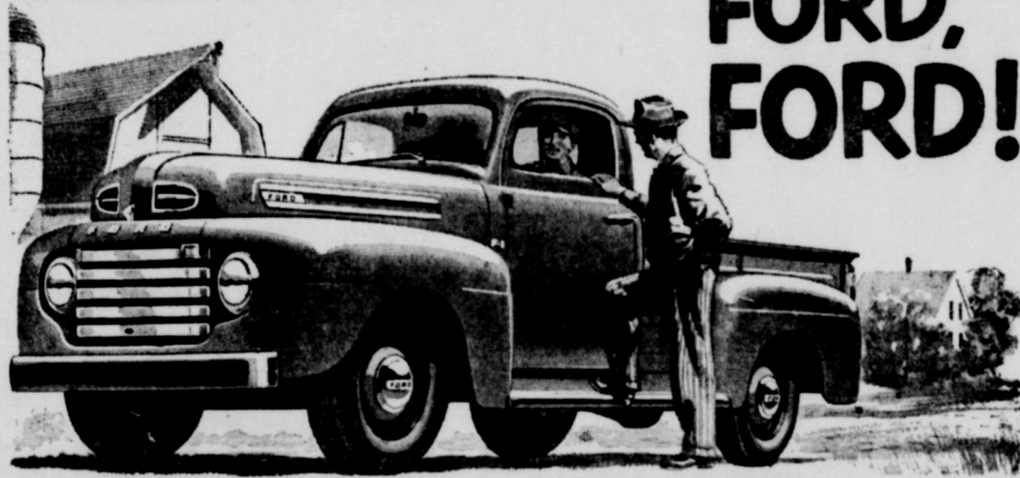
#16, 17 Ford F-1 Pickup shown here, C.V.W. rating—4,700 lbs. Body capacity—45 cu. ft. Available with 35-h.p. Six or 100-h.p. V-8. Use of over 175 models including 145-h.p. Big job.
