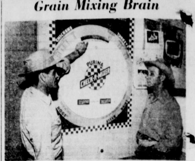
A "grain mixing brain," which calculates the exact amount of concentrate needed to balance out any given amount of ground home-grown grains for most economical production of meat, milk or eggs, has been obtained by the Kemp Feed and Hatchery in Ballinger, from the Ralston Purina Company in St. Louis. The device, known as the "Checker-R-Mixer" has been installed in the grinding and mixing mill and is now in use. It is built in the form of a large dial. In using it, the mixer operator determines the amount of grain the farmer has brought in, then dials that amount to the section for chickens, turkeys, hogs, cattle or dairy cows, depending on what kind of feed is being mixed. The dial reading then shows the exact amount of supplement to be added to the grain. Although 97,000 different formulas can be calculated on the Check-R-Mixer, its calculations vary less than 1/2 of one per cent from Purina research formulas, leaving practically no margin for error in computing the best mixture of grains and supplements.
