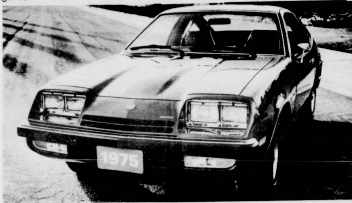
The soon-to-be-introduced 1975 Monza 2+2, Chevrolet's new sporty European-type compact, is a four-passenger hatchback sportster that has two bucket seats in the front and seating for two in the rear. The rear seat can fold into a cargo area. Front lighting on the Monza 2+2 is new with the first usage of dual rectangular headlamps (lower left). Parking and turn signal clear lens lamps are mounted in the lower valance panel. Wrap-around rear lighting units (lower right) provide for all rear lighting requirements. Rear panels, like the front, are soft faced with integral bumper guards and a full-width bumper strip.
