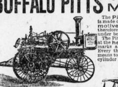
The Pitts Traction Engines are recognized as being at the head of the list, but the Double Cylinder marks a new era in Traction Engine building. Every thresherman will at once recognize what it means to have no dead center. We also have single cylinder Engines for those who desire them.
