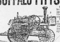
The Pitts Double Cylinder Traction Engine is made on the same principle as Railroad Locomotives, two cylinders being used side by side, therefore no dead centers either on the road or
