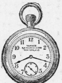
The Yankee Watch movement is size 1 in diameter and % of an in in thickness. Lantern pinions, American lever, patented lever escapement, 240 beats per minute. Polished
