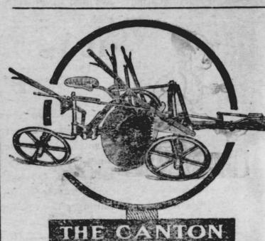
The P. & O. Canton No. 3 Disc Plow is unrivaled in strength. It has all the ad uniments accessary for all conditions under which a disc plow must work. The controlling rod regulates the rear wheel, the course of the plow can be changed without stopping the team, and the rear wheel is not influenced by the movement of the team or irregularities of the land. The width of the furrow is fixed by the front furrow wheel lever.
