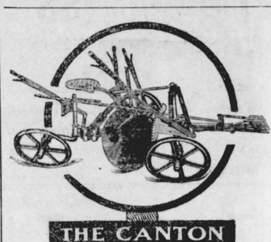
ularities of the land. The width of the furrow is fixed by the front furrow wheel lever. The scraper can be set to any desired pitch or angle and is a positive disc clear elso assists in cleaning the furrow properly. The disc is ball-bearing and dust-proof and revolves freely from the slightest contact with the ground.
