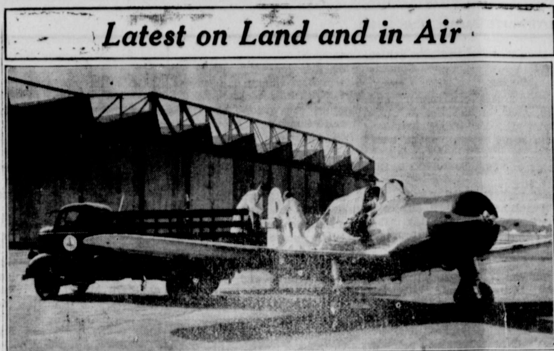
Latest on Land and in Air The up-to-the-minute monoplane being serviced by the Chevrolet truck above is the new Vultee Valiant 54, a basic training airplane built by Vultee Aircraft, Inc., which also produces pursuit planes and bombers. The craft has a 42-foot wing-spread, and when loaded weighs just under two tons. It has a cruising range of 1,050 miles, a service ceiling of 21,000 feet, and a landing speed of 53 miles an hour. Both plane and truck, of course, have valve-in-head engines for the maximum dependability and power which that type of power plant provides.
