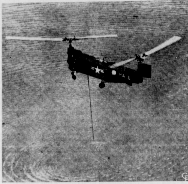
UNDERWATER snooping technique is demonstrated by the Navy's new anti-submarine helicopter as it hovers motionless over the water near Fort Worth, Tex., with its latest dipping sonar detection equipment under the surface. The 'copter carries "homing weapons," which basically are lightweight torpedoes containing target-seeking guiding mechanisms to seek out and destroy enemy undersea craft far below.
