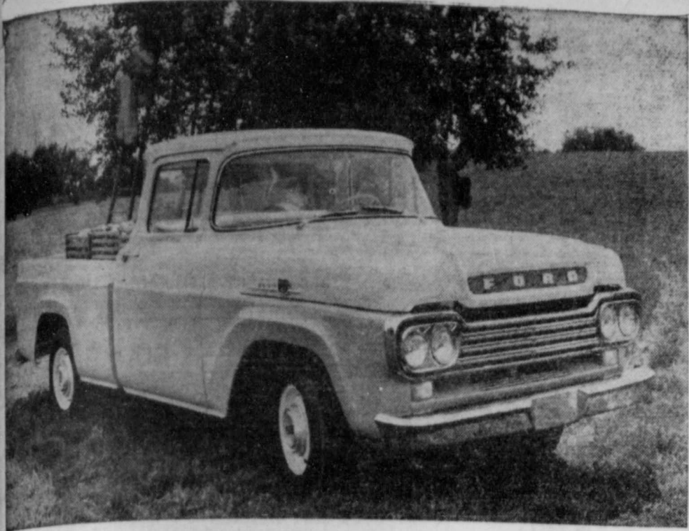
The popular F-100 pickup is one of 371 Ford truck models available in 1959. Dual headlights and a new Ford nameplate on the hood are standard features on the pickup models. With the 223 cubic inch six-cylinder engine — the most modern "six" in the industry — Ford offers greater economy in the high speed or increased load range. The pickup is available with either this desirable body, which Ford pioneered with the 1957 models, or the Flareside body. The 1959 Ford truck line is now on display at Edgington Motor Company in Goldthwaite.
