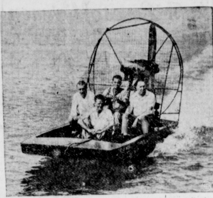
SKIMMER TO THE RESCUE —As the nation's foremost disaster fighter, the Red Cross uses many of science's latest inventions to gain speed and mobility. This new gimmick was developed by the Dade County, Fla., Red Cross chapter for water rescue work. Driven by airplane propellers, the flat-bottomed boat will travel 50 miles an hour in only six inches of water.
