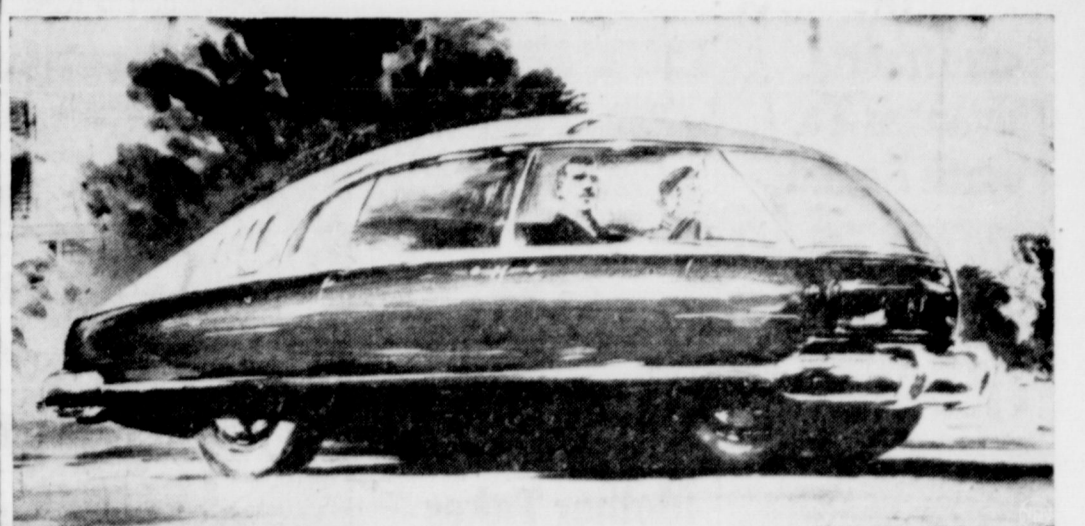
"TURBOCAR" IN YOUR FUTURE—This is what your "turbocar" of the future will look like, according to British jet expert G. Geoffrey Smith. The design promises greater visibility and more body space thanks to the gas turbine power unit located over the rear axle.
