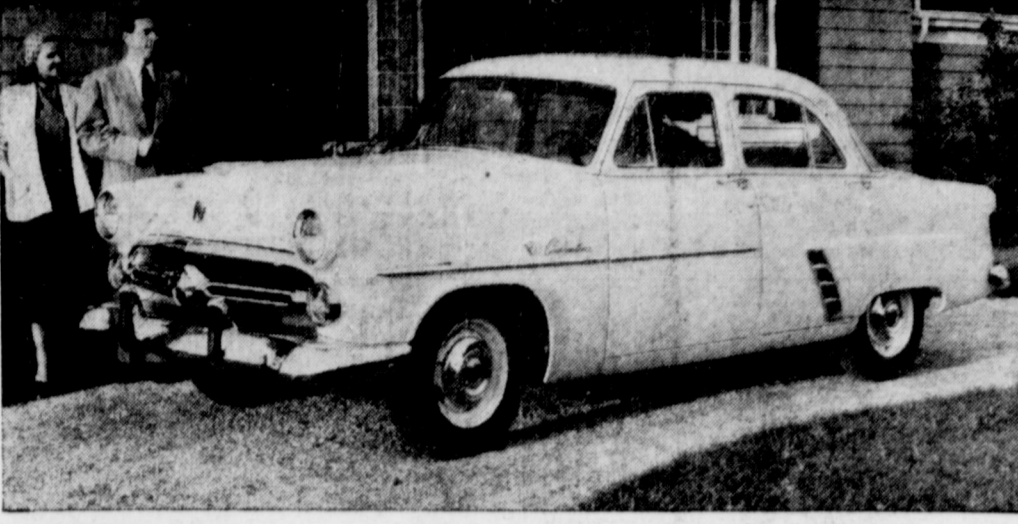
The all-new 1952 Ford Customline Fordor Sedan features a completely new Ford Coachcraft body with curved one-piece windshield and rear window, triple-spinner grille arrangement and body highlights sweeping backward from the extended headlights along the hood and fender to the jet-tube taillight sections. Added styling features of the Customline Fordor are the chrome capped rear fender profiles.
