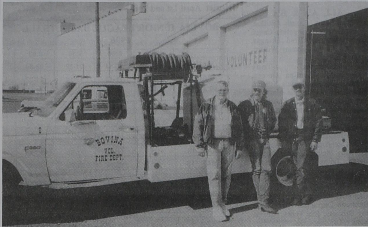
NEW FIRE TRUCK..... Pictured with the newest addition to the Bovina Fire Department are l-r, Chief Richard Bonham, Stan Miller, and Jessie Stone. The truck was donated by the County Precinct 2, and the 450 gallon tank was given by the school district. Miller and others did the refurbishing of the 1984 Ford, F350 truck, which has a generator on the rear that can be used for lighting.
