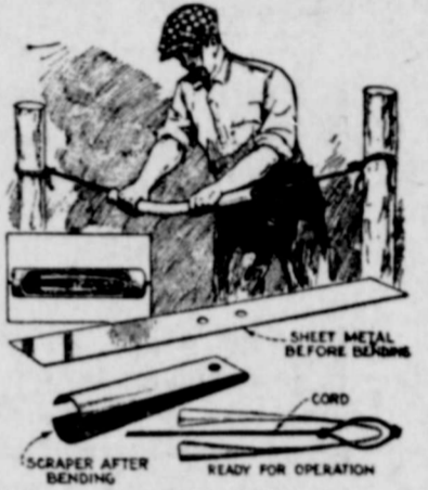
Simple Device for Scraping Carbon From Exhaust Pipes.
