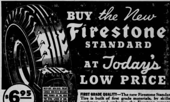
FIRST GRADE QUALITY-The new Firestone Standard Tire is built of first grade materials, by skilled workmen, and embodies the Firestone patented construction features of Gum-Dipping and two extra layers of Gum-Dipped cords under the tread. GUM-DIPPED CORD BODY-Every cotton fibre in every cord in every ply is soaked in liquid rubber.
