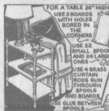
FOR A TABLE 26" HIGH USE 3 BOARDS WITH HOLES BORED IN THE CORNERS USE 52 SMALL SPOOLS AND 24 LARGE ONES USE 4 BRASS CURTAIN RODS RUN THROUGH SPOOLS AND BOARDS USE GLUE BETWEEN SPOOLS
