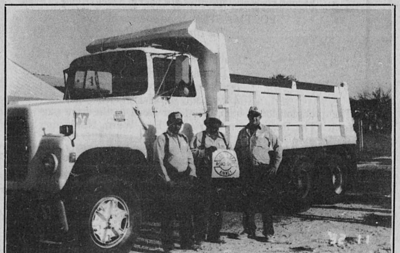
New Dump Truck: Road Administer Cliff Fritter, right, and Judge Tim Ward went to Fort Worth late last week and purchased this 1985 Ford 8000 dump truck, 14 yard bed, for the county road department. With Fritter are road department employees Armando Sanchez and Caesar Daniels. This truck will more than double the load capacity of the two old trucks.
