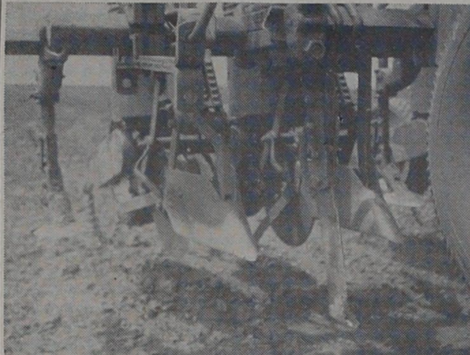
One row of the four row implement shows the attachments on the three tool bars. In front is the ammonia chisel, next are two bead cleaner sweeps that open the water furrow.
