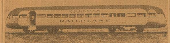
ly streamlined railroad coach, according to statement of its designer, William B. Stout. The bulletshaped car, which receives its power from two automotive type engines, one driving the front axle and the other the rear axle, has been tested at the Dearborn, Mich., track. It was built for the Pullman Car & Manufacturing Corporation
