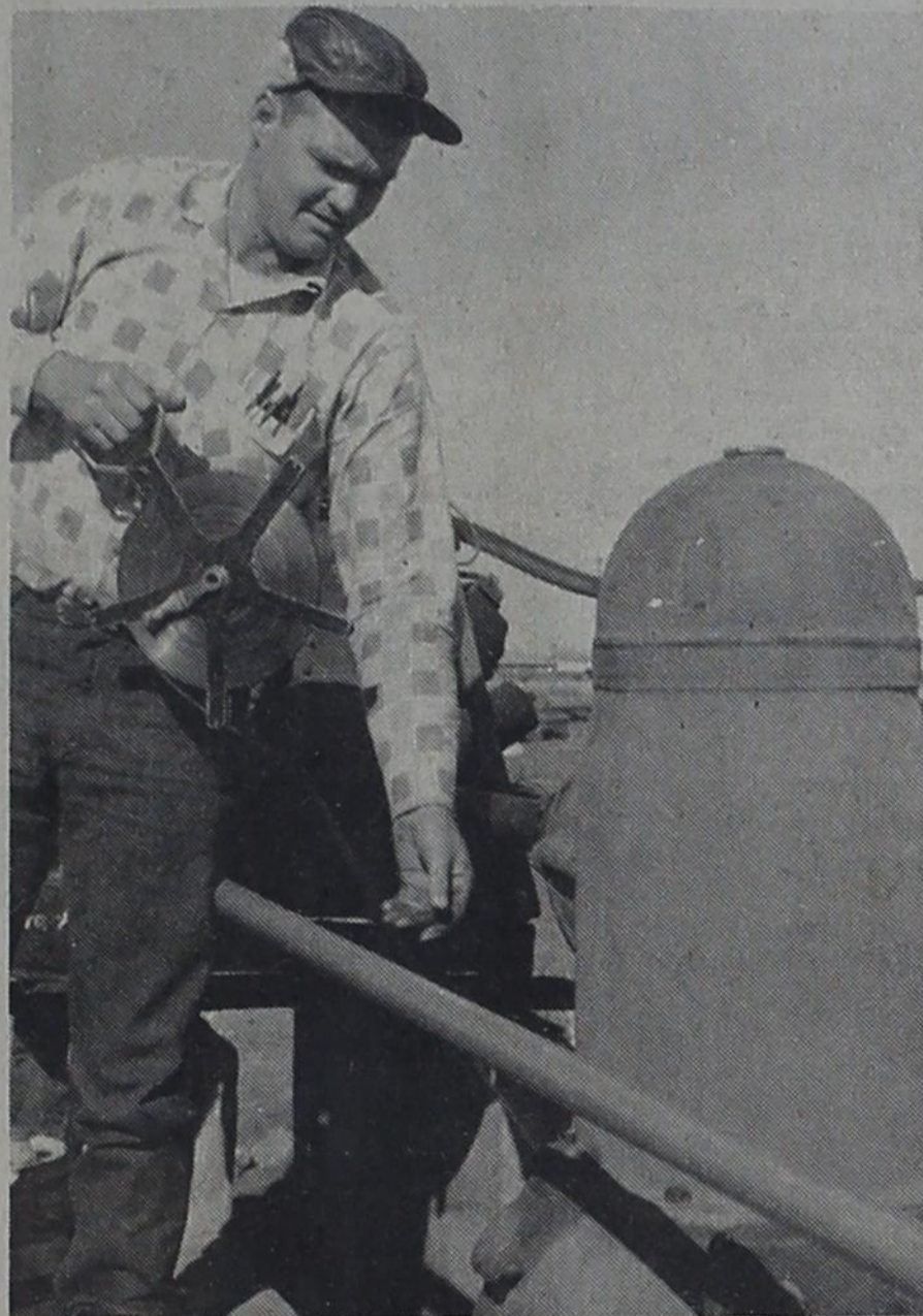
PAUL RETTMAN of the U. S. Geological Survey takes a measurement to the water table of a Farmer County irrigation well. He runs in enough steel tape down the side of the casing to reach to the level of the water. The way he determines the level is to subtract the amount of tape found to be wet when the tape is reeled back up, from the amount of tape that was rolled down into the well.
