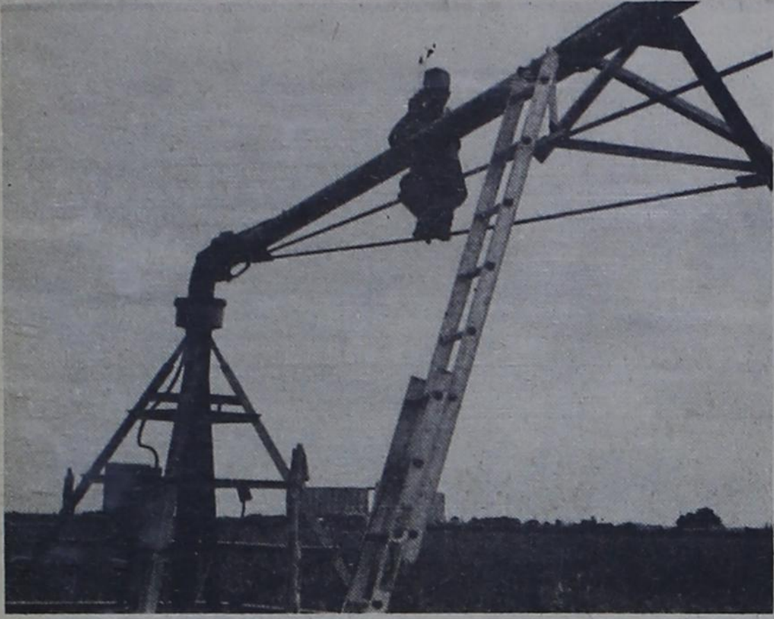
WATER FLOW CHECKED.... During a center-pivot sprinkler evaluation the water flow into the system is checked with a velocity meter. Henry Skala, SCS employee, is shown reading the Cox velocity meter.
