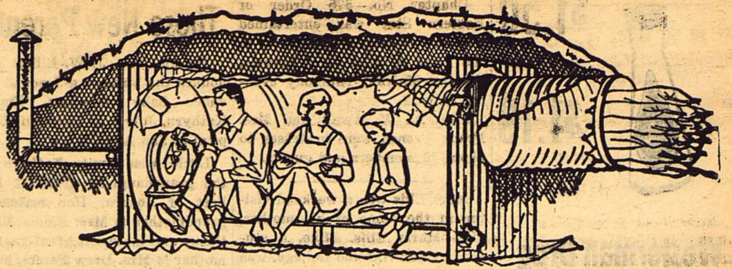
PRE-FAB corrugated steel culvert fallout shelter for three persons can be bought for about $150, plus delivery and installation. The shelter, which would cut to 1/500th the amount of outside fallout radiation exposure of its occupants, is included in the "Family Shelter Designs" booklet now at state and local civil defense offices for public distribution. It is available without charge.
