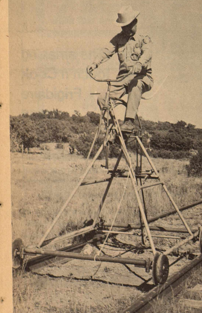
THIS INTERESTING APPARATUS was discovered recently by Nolan Johnson, local game warden. The bicycle like vehicle had apparently been used for illegal hunting from the railroad track. Apparently home made, the unusually quiet four wheeler ran along the tracks with little effort by the operator and being high above the ground should make that buck an easy target. According to Johnson, he and other game wardens have been seeking the owner or owners of the clever machine for several nights, to no avail. Johnson added that the owner may claim his vehicle by contacting either him or the railroad.
