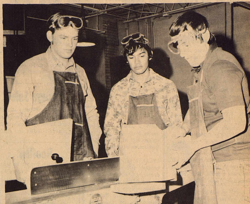
Students in Shop I learn the use of a joiner machine in building their project. Safety glasses are used for the boy's protection. Left
