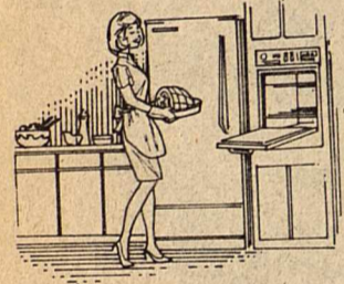
DON'T INSTALL a built-in oven without counter space alongside. You need a place to rest prepared food while loading or unloading the oven.
