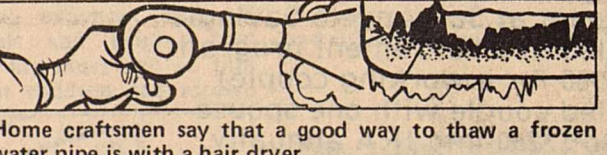
Home craftsmen say that a good way to thaw a frozen water pipe is with a hair dryer.
