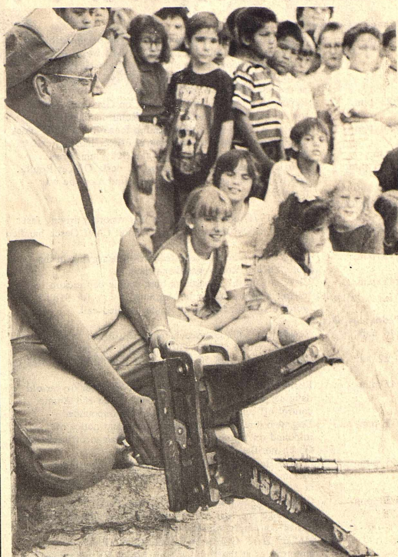
Jaws of life-Louis Olenick demonstrates how the jaws of life extrication device is used by fire fighters to free victims in automobile accidents. The fourth graders were given demonstrations in various rescue techniques.
