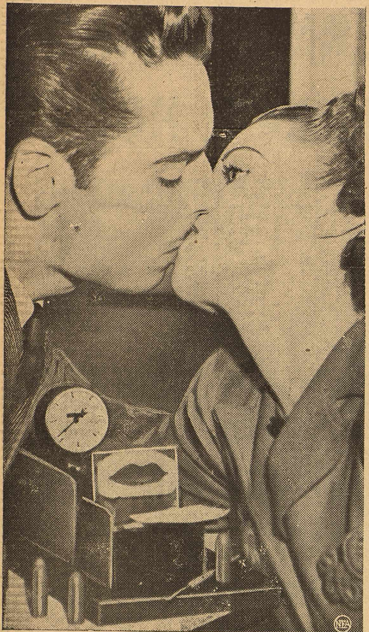
Lazy lips lost a pleasant job for Bob Roberts and June Baker, professional kissers, above. When they couldn't keep up the required 10 pounds pressure for each smack in testing lipstick, a mechanical applicator, center, took over their work. The kissing machine pumps two sets of lips in firm contact to leave lipstick imprints on paper placed between them.
