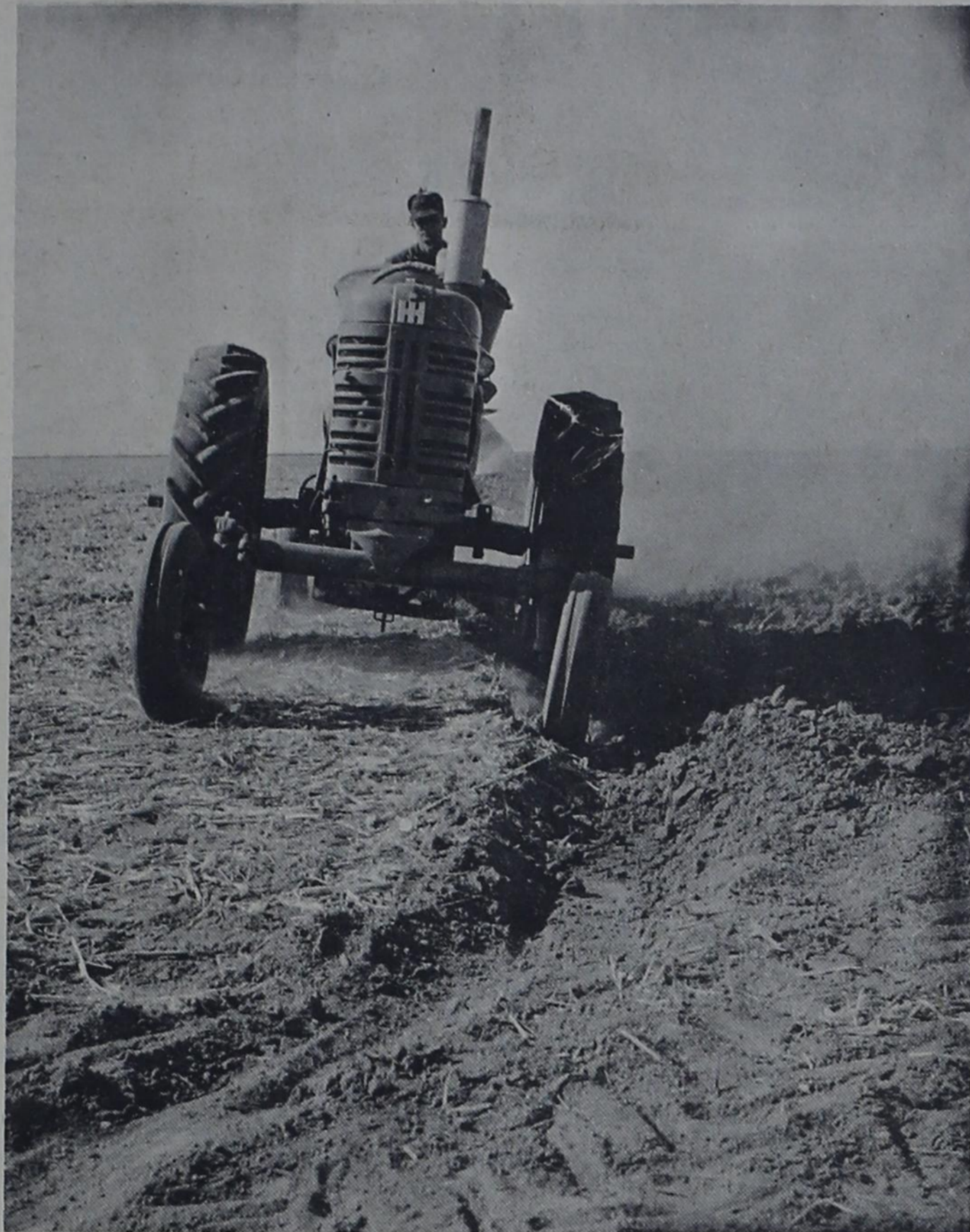
The two-way or "roll-over" plow is utilized to good advantage by many High Plains farmers, especially when they do such fall plowing as is shown above. In the left picture the tractor is headed east. In the right picture it's headed west after the driver has turned around and "rolled" his
