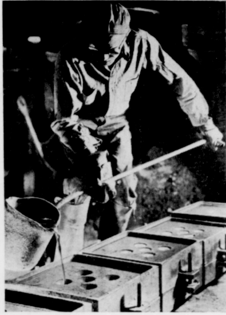
Aluminum is used in countless forms—sheet, tubing, forgings, extruded shapes, impact extrusions, foil and wire, to name a few. This workman is pouring small sand castings.
