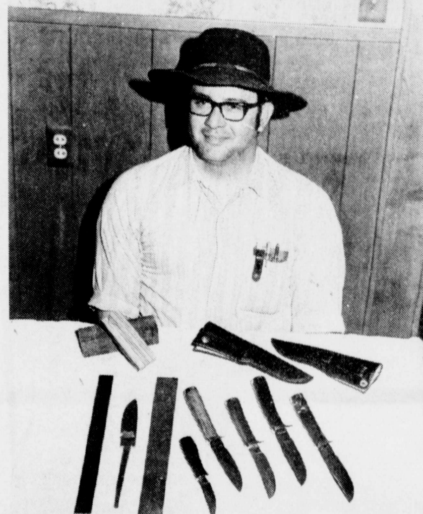
The process begins with the steel being forged to shape with a hammer and anvil. The blade is then rough ground on a belt grinder that runs 4700 sanding feet per minute on an 8" cog wheel. After the shaping, the blade is put back into the forge, heated and oil hardened, then hand tempered with hot tongs to achieve the proper hardness. Three degrees of hardness are put into each knife to insure strength, and maximum edge-holding ability.
