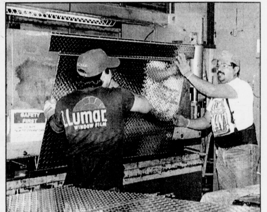
JOHN'S INTERNATIONAL EMPLOYEES Omar Armendariz (left) and Renaldo Ramos form the wrapper which is the bottom part of the full size diamond aluminum plate truck box. Armendariz has been with John's for about a year and Ramos two years.
